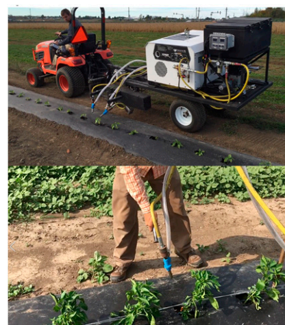
Fig. 1. Prototype abrasive grit applicator (top image) with air compressor (white), fertilizer grit hopper (black), compressed air and grit delivery tubes (yellow and white, respectively), and prototype grit delivery nozzles (blue and metallic); and a hand-held application of organic fertilizer grit in pepper planting holes in this study (bottom image).
