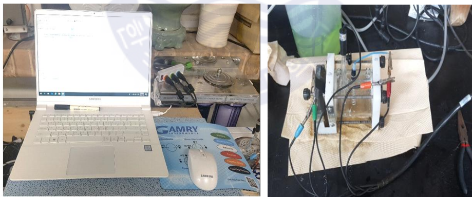
Fig. 3.7 Measuring views of electrochemical anodic polarization test
