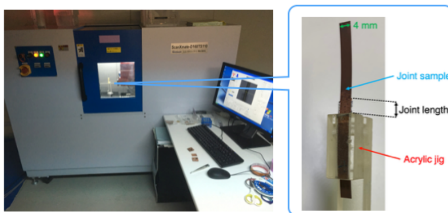
Fig. 4.7: Experimental set up for X-ray CT scan
