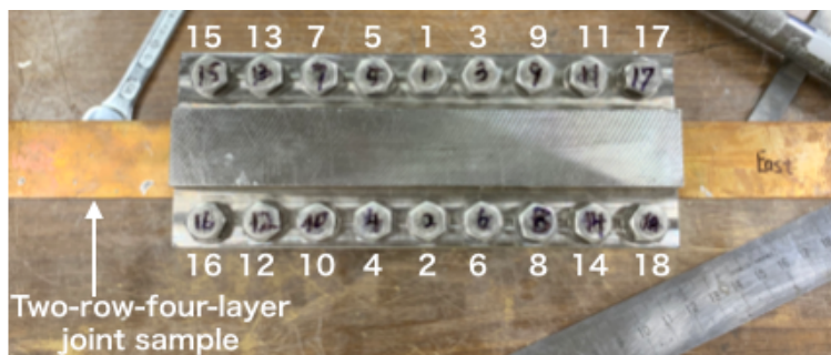
Fig. 5.10: Sequence of bolting
