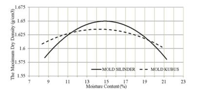
Figure 7: The Comparison Soil Compaction Modified Proctor
