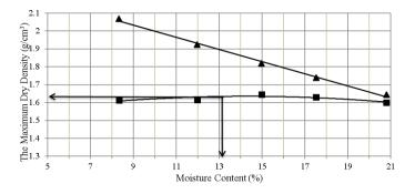
Figure 5: The Relationship of Dry Volume Weight and Moisture Content of Soil Compaction Modified Proctor
