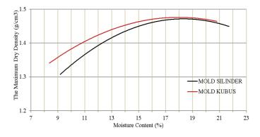
Figure 6: The Comparison Soil Compaction Standard Proctor Collision Method Using Cylindrical and Cube Mold
