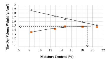
Figure 4: The Relationship of Dry Volume Weight and Moisture Content of Soil Compaction with Standard Proctor
