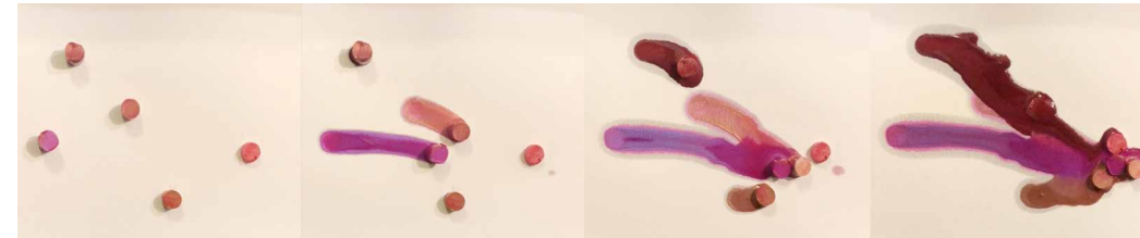
Experiment 2.3 - 6 Lipsticks w/. Tilted Surface and Single Side Heating
