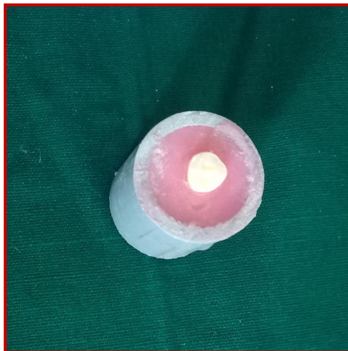
Fig 14. Teeth embedded in self curing acrylic resin blocks
