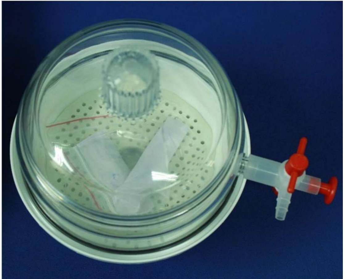
Fig 5: Silver coated wires in vacuum desiccator
