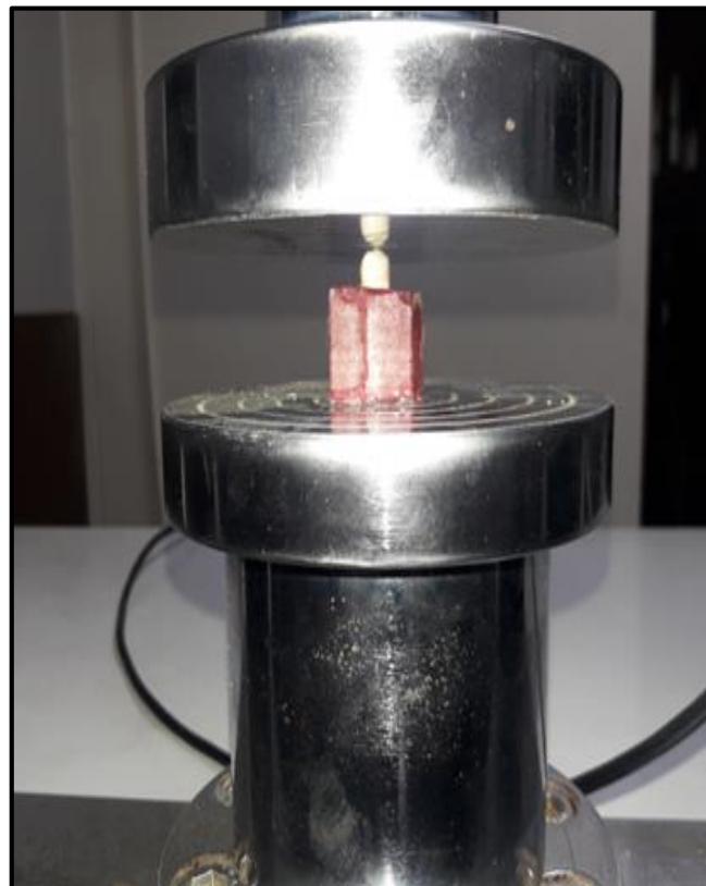
Fig 10: Fracture toughness testing
