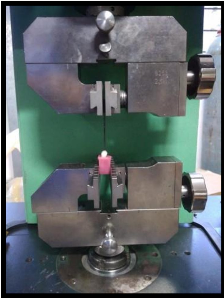
FIG 12 : TEETH SAMPLE MOUNTED ON UNIVERSAL TESTING MACHINE FOR FRACTURE TESTING
