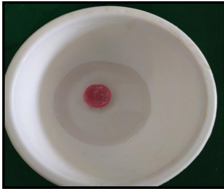
Figure 11 : Immersing in the second test solution for 5 minutes
