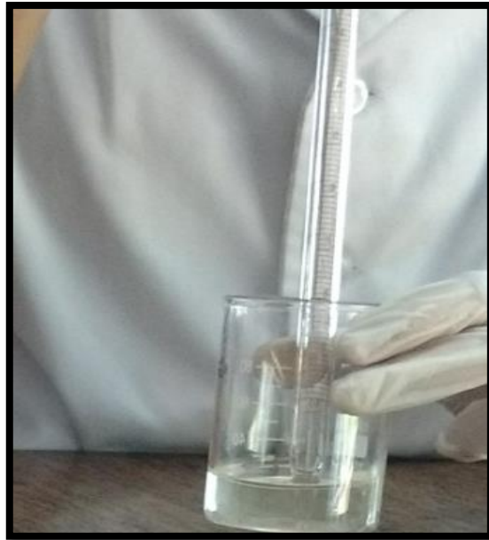
Figure 8: 10 ml of test solutions were pipetted
