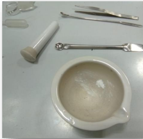
Fig 3.2 Potassium bromide addition to the fine powdered sample
