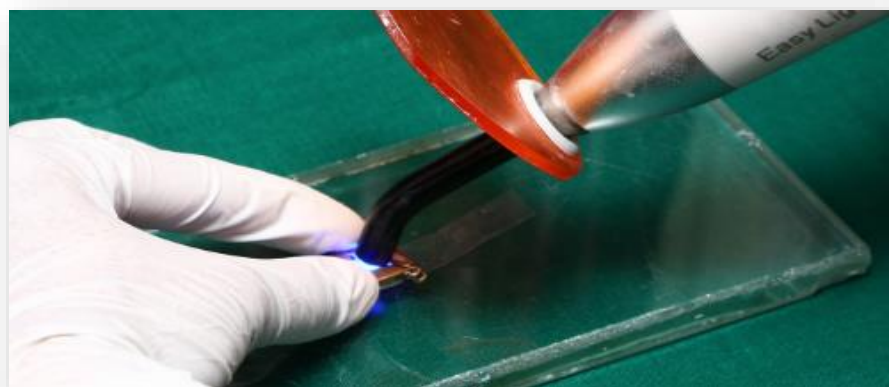
Fig 2.2 Light curing of composite block
