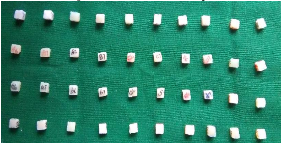
Fig 2.3 Tetric N Ceram bulk fill composite blocks
