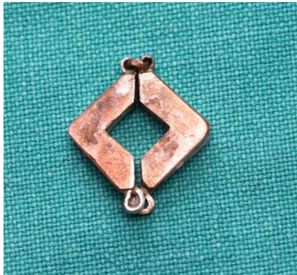
Fig 1.1 Split mold of length 5 mm × width 5 mm × height 3 mm
