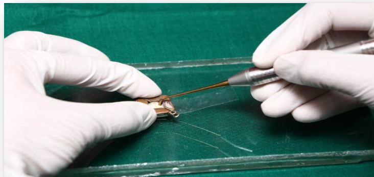
Fig 2.1 Placement of composite into the mold
