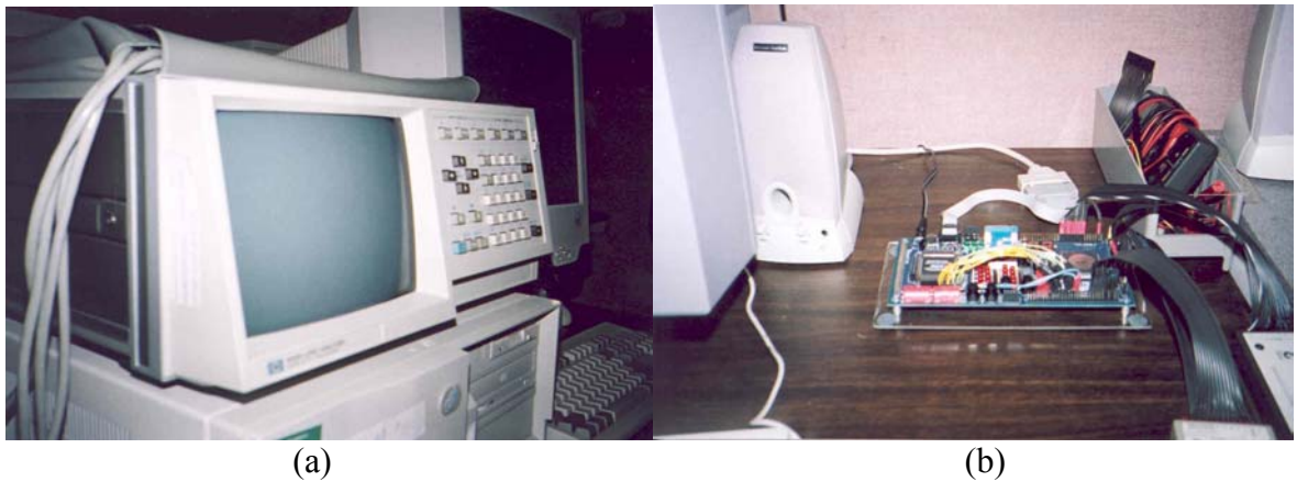
Figure 5-3. Microdot FPGA Test Setup. Included (a) HP1630D Logic Analyzer and (b) Altera UP-1 design board
