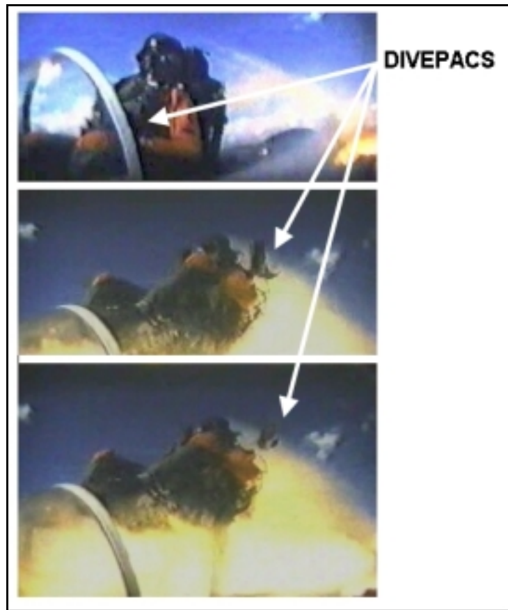
Figure 57. Manikin Entering Airstreams, HMTT, 31 Oct 01
