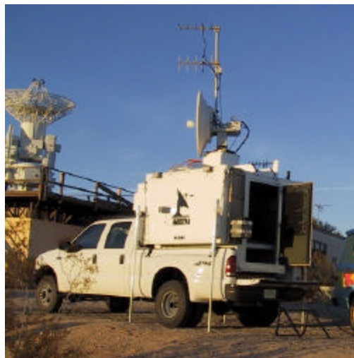
Figure 26. S250 Comm Shelter
