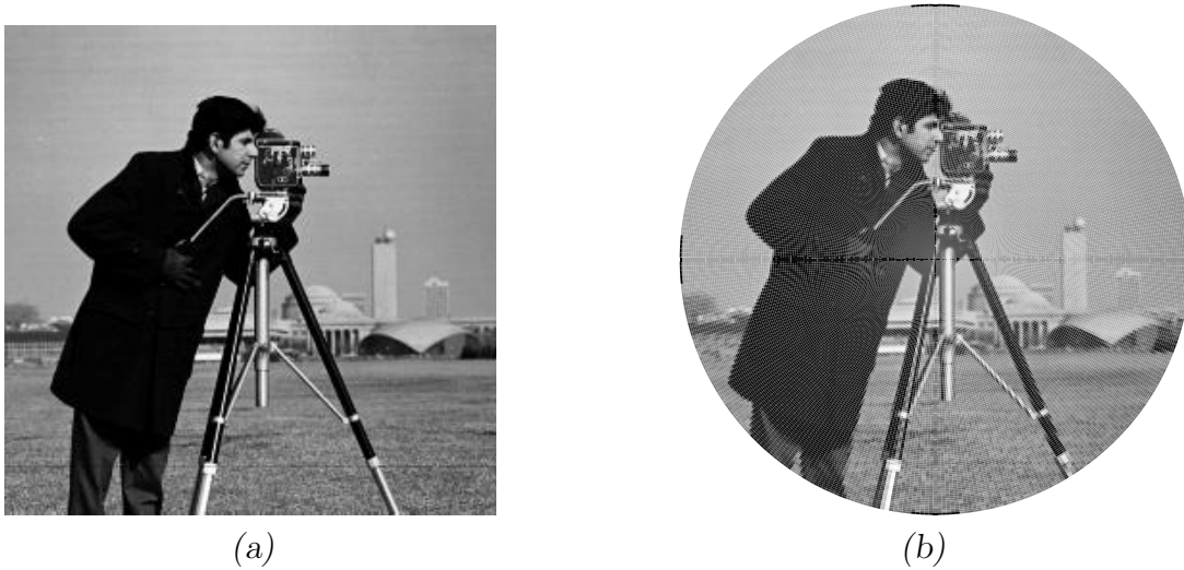
Figure 3.5. Converting Cartesian Coordinates to Polar Coordinates. (a) Camera-man image in Cartesian coordinates. (b) Cameraman image in polar coordinates.
