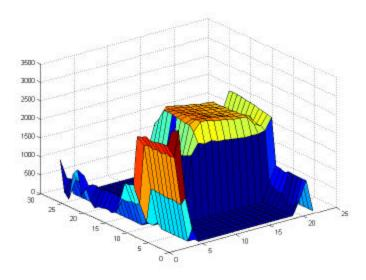
Figure 28 Coarse estimate of the very-low dose (50 mRad) image found by creating a background consisting of  $200 \times 200$  blocks with vertices corresponding to the minima of the  $200 \times 200$  blocks of the original image
