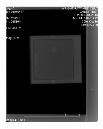
Figure 14 Medium-high dose mammography image of the American College of Radiology (ACR) phantom captured at 125 mRad. Evidence of low contrast, scattering, and noise degradation continues to be apparent.
