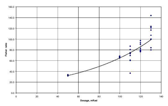
Figure 90 Comparison of Fisher ratio for the contrast of the disk and the background of the Post-processed image for various doses of X-rays.
