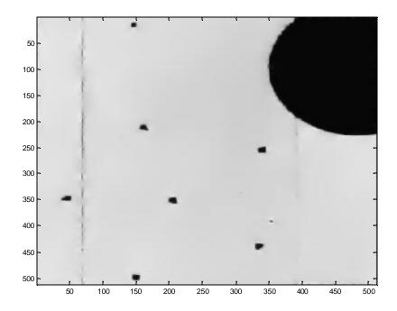
Figure 35 uneven illumination corrected, histogram equalized, RDWT denoised very-low dose (50 mRad) image.
