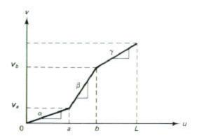
Figure 2 Non-linear function to perform contrast stretching. Here u represents the given pixel gray level and v is the mapped output pixel gray level. The variables  $\boldsymbol{a}$ ,  $\boldsymbol{b}$ , and  $\boldsymbol{g}$  represent the slopes of the transformation function respectively, L represents the maximum given pixel gray level, and a and b represent the variable parameters for the start and finish of the region of stretching (11:235).
