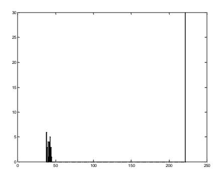
Figure 88 Histogram of 60 pixel values (30 inside and 30 just outside of the disk, chosen randomly using IMPIXEL) for the post-processed High dose (130 mRad).
