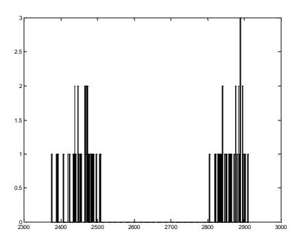
Figure 78 Histogram of 60 pixel values (30 inside and 30 just outside of the disk, chosen randomly using IMPIXEL) for the Very-low dose (50 mRad) image.
