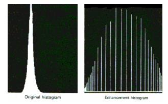
Figure 3 Original histogram is from the original image and enhancement histogram is from the image after contrast stretching. Contrast stretching spreads a "peaky" histogram by multiplying the pixels corresponding to the "peaky" portion of the histogram by the high slope portion of the non-linear function (11:236).
