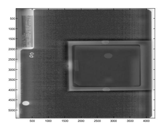
Figure 70 Uneven illumination corrected High dose (130 mRad) image.
