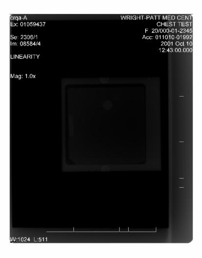
Figure 12 Low dose mammography image of the American College of Radiology (ACR) phantom captured 75 mRad. Evidence of low contrast, scattering, and noise degradation is apparent.
