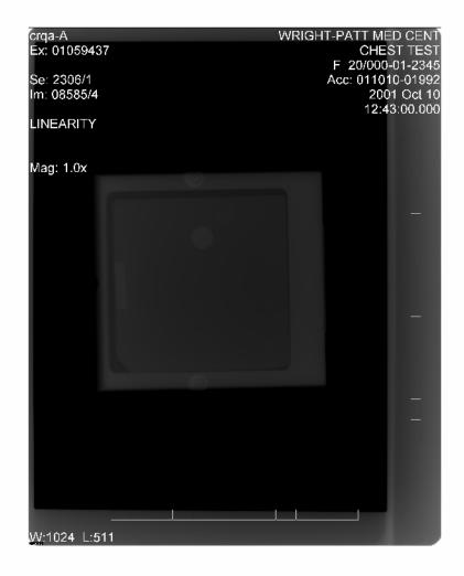
Figure 13 Low-medium dose mammography image of the American College of Radiology (ACR) phantom captured at 100 mRad. Evidence of low contrast, scattering, and noise degradation is still apparent.
