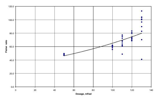
Figure 103 Comparison of Fisher ratio for the contrast of the specks and the background of the Post-processed image for various doses of X-rays.
