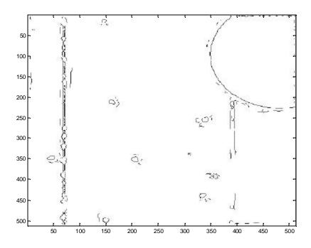
Figure 36 Edge detected post-processed very-low dose (50 mRad) image using the Canny method.
