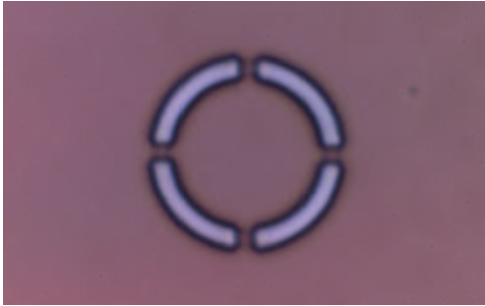
Figure 4.5 Microscope view of device oxidation etch holes. After etching by RIE, the \text{Al}_{0.98}\text{Ga}_{0.02}\text{As} layer is exposed and oxidized in water vapor. The resulting oxide aperture acts as a current funnel for the VCSEL.
