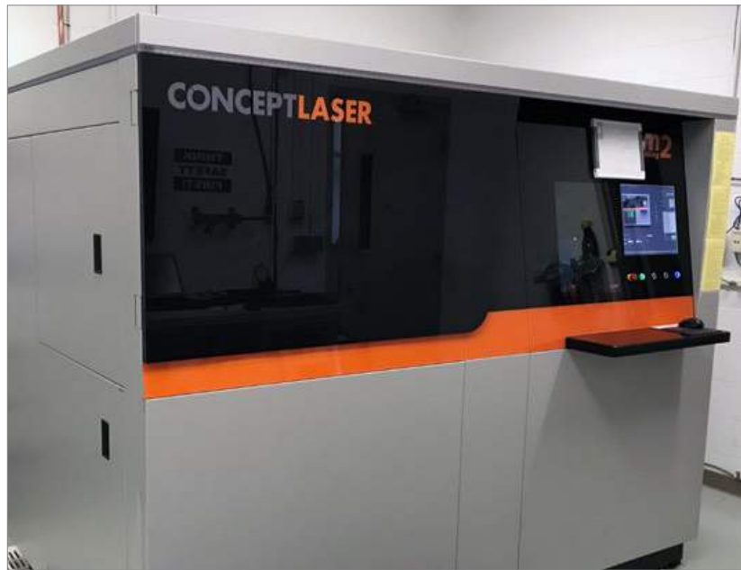
Fig. 6 AFIT's M2 Cusing metal Additive Manufacturing system
