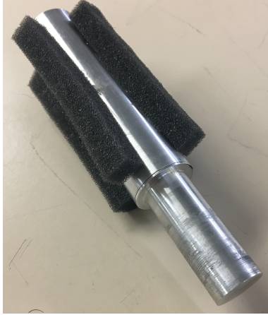
Figure 6.4. The \text{LaBr}_3(\text{Ce}) detector with integrated PMT and foam supports. The active part of the crystal is contained in the smaller aluminum housing in the lower right hand corner of the photo.
