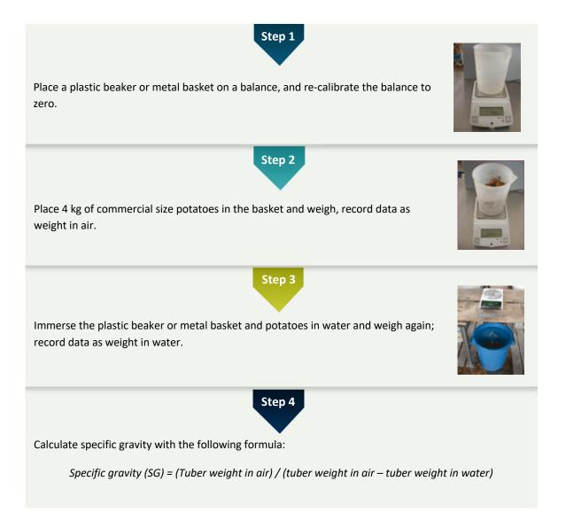
B. - Determining specific gravity with the hydrometer method
