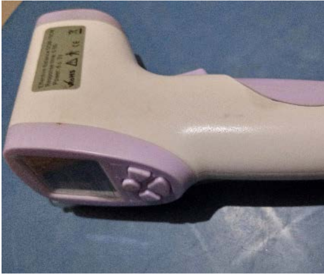
Figure 9: Infra-red digital thermometer. Credit: CIAT/P. Zaake
