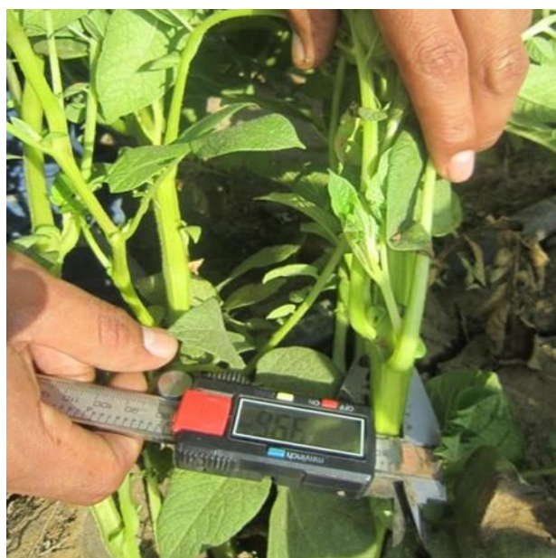
Fig.5 Correct stem diameter measurement example.
