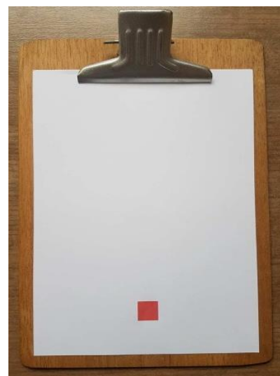
Fig. 9 Example of a fabricated picture table for determination of Leaf Area.
