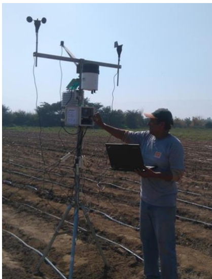
Fig. 1 Hobo U30 complete weather station.
