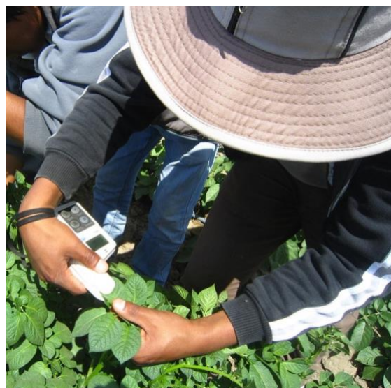
Fig. 8 SPAD equipment. Showing the correct position of usage.
