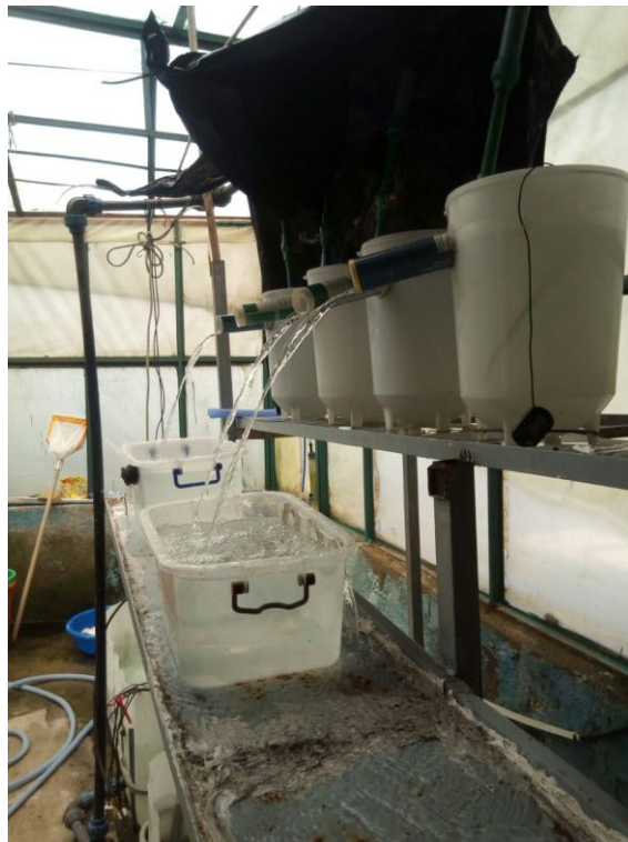
Figure 4. Recirculating aquaculture system for hatching Nile tilapia
