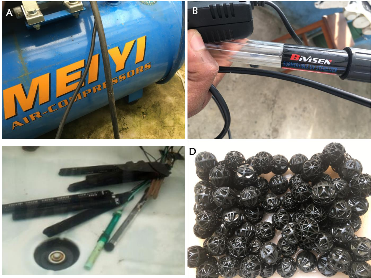
Figure 2. Equipment for maintaining water quality parameters in the system (air compressor (A) ultraviolet (UV) lamp (B), heaters (C), bioballs (D))
