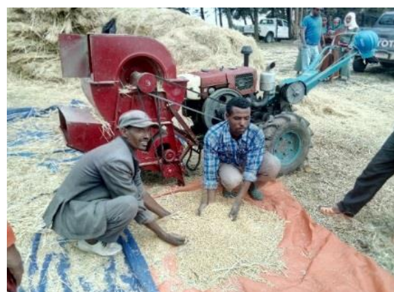
Photo 1: Two-wheel tractor powered wheat threshing and maize shelling provided by service providers in rural communities of Ethiopia (photo credit: CIMMYT/Walter Mupangwa)
