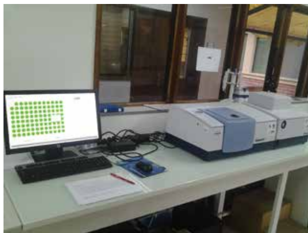
The Fourier-transform infrared spectrometer Tensor 27 (Bruker Optics, Karlsruhe, Germany) with a high-throughput screening extension unit used for the near- and mid-infrared light soil analyses
