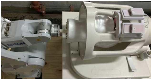
Fig. 1. Out-of-bore experimental setup: Epson C3 6-axis robot used to control the pose of a polystyrene head phantom inside an 8-channel head coil; custom bracket for mounting two MR-compatible cameras to the coil for prospective motion correction.
