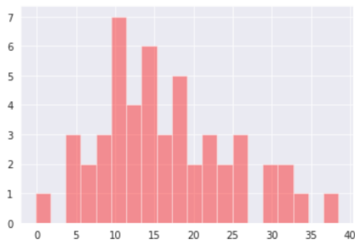
Figure 9.11: Histogram of percentage reductions of maximum running time (in seconds) on the 50 random graphs between the benchmark and our pruning methods for failure cases. These values indicate that our pruning method is better than the benchmark method in terms of maximum running time.
