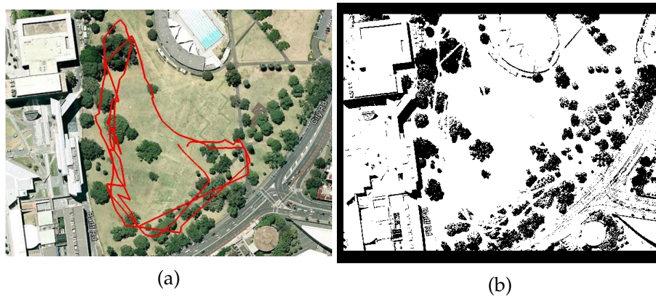
Figure 6.3: The Victoria Park grid map. (6.3a): A plan view of the Victoria Park terrain [39]. (6.3b): An occupancy grid map of the Victoria Park terrain.
