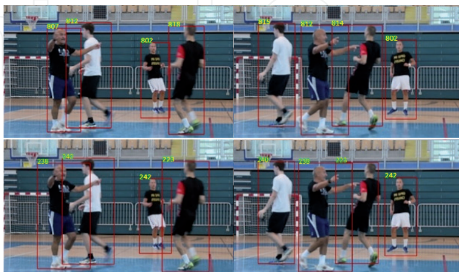
Figure 6. An example of tracking situation with occlusion. Top: Hungarian algorithm, bottom: Deep SORT. The left and right frames are 1 second apart.
