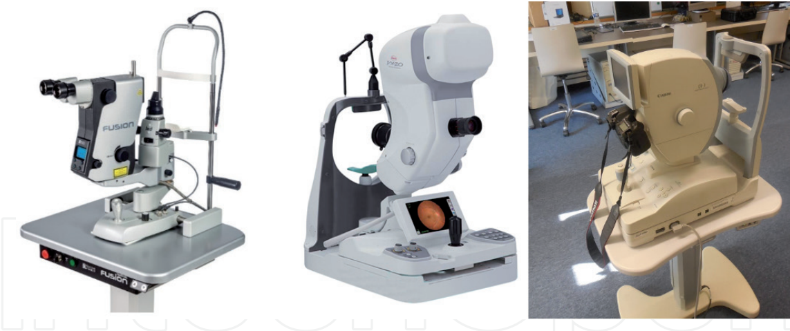
Figure 3. Slit lamp example (left) [6]; example of a non-mydratric fundus camera (middle) [7]; (right) fundus camera used in the biometric laboratory at FIT BUT (right).
