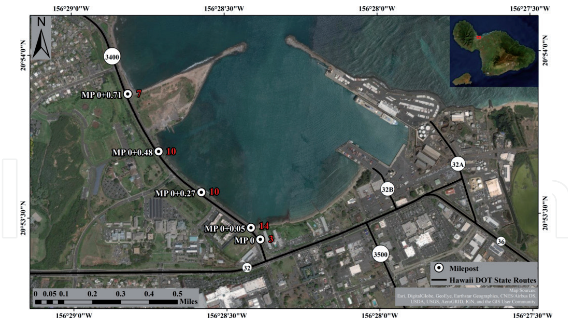
Figure 20. Ocean Hazards Classification Scheme (OHCS) ranking for Maui Central Maui (CM) MP 0 to 0 + 0.71. The OHCS consists of five variables: (i) sea level rise 1905–2050, (ii) maximum annually recurring significant wave height 2010–2018, (iii) shoreline change 2008–2100 and CRESI Armoring, (iv) historical and hypothetical tsunami, and (v) Category 1,2,3,4 hypothetical storm surge. Rankings of ocean hazard increase from 1 to a theoretical maximum of 100.
