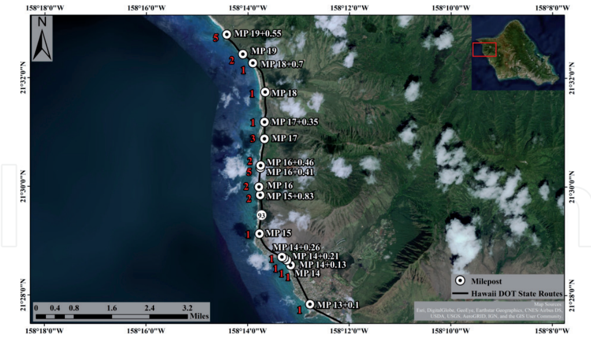
Figure 2. Ocean Hazards Classification Scheme (OHCS) ranking for Oahu Waianae Coast (WC) MP 13 + 0.1 to 19 + 0.55. The OHCS consists of five variables: (i) sea level rise 1905–2050, (ii) maximum annually recurring significant wave height 2010–2018, (iii) shoreline change 2008–2100 and CRESI Armoring, (iv) historical and hypothetical tsunami, and (v) Category 1,2,3,4 hypothetical storm surge. Rankings of ocean hazard increase from 1 to a theoretical maximum of 100.
