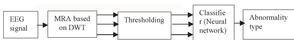
Figure 14. Wavelet based EEG signal classification system.
