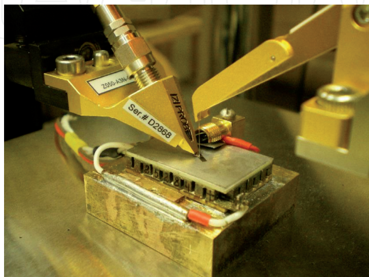
Figure 3. The workbench for VCSEL chip's study.
