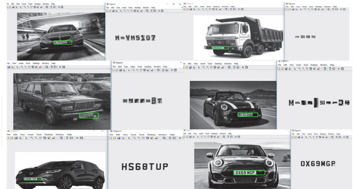
Figure 6. The results for objects with number-plate.
