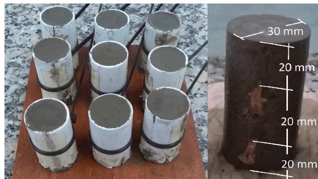
Figure 5. Molds and dimensions of cement cylinders.
