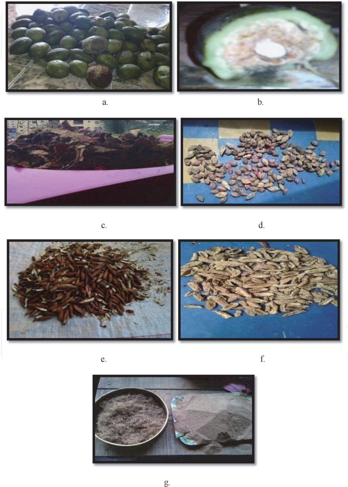
Figure 2. Sea almond fruit biomass, a. the fruit, b. fruit cut section, c. dried fruit pulp, d. inner seed with coat. e. the seed, f. the fruit husk, g. the ground pulp (raffinate and 600 \mu\text{m} particle size).
