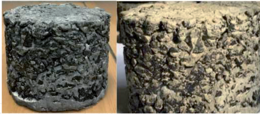
Figure 2. Disconnectivity of internal voids due to low air-voids [18].
