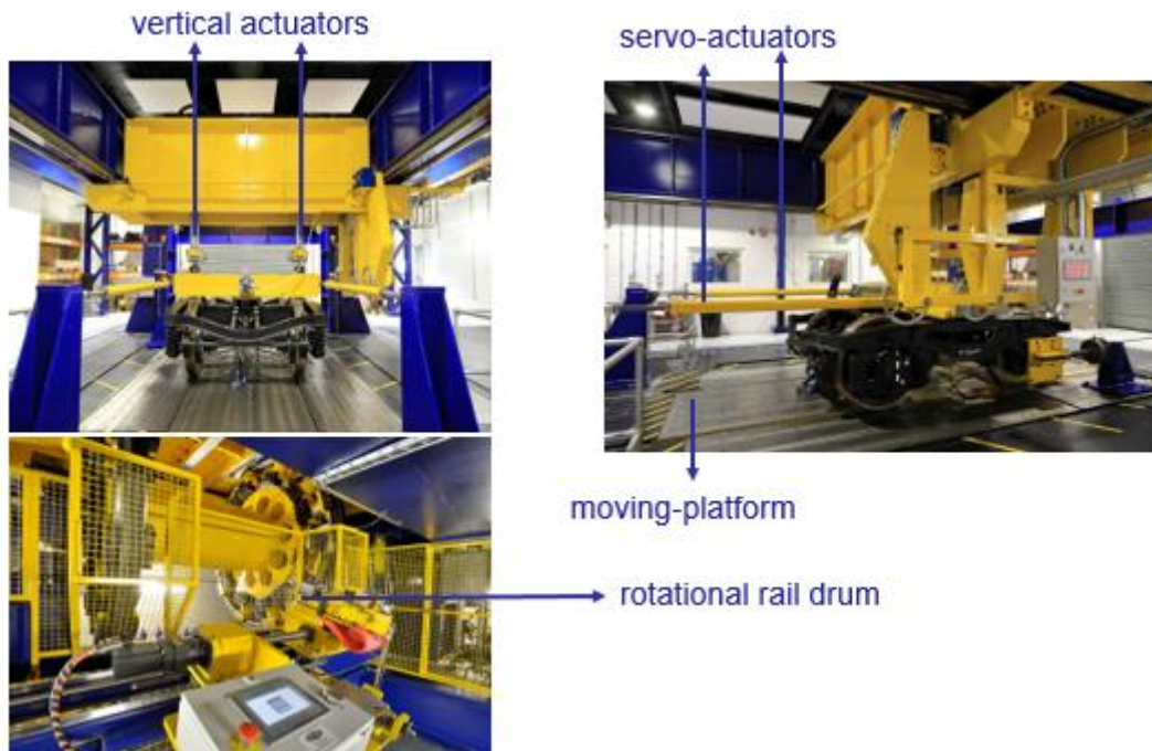
Figure 1: Full scale HAROLD test rig with its components
