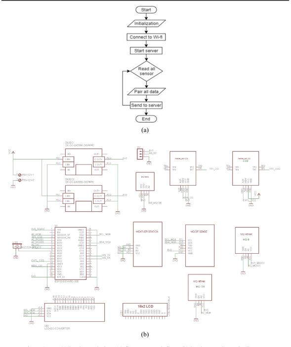
Figure 2. ESP32 hardware design: (a) firmware work flow, (b) hardware schematic diagram
