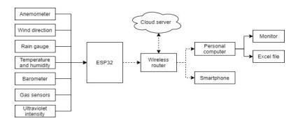
Figure 1. System block diagram of the weather station
