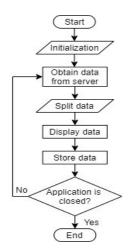
Figure 3. Weather station desktop application software work flow
