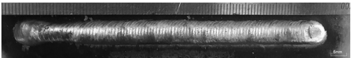
Figure 102 The welding layer with 7.5m/min of feeding wire speed
