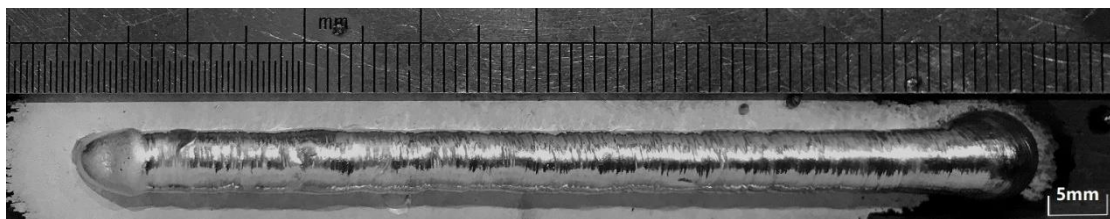
Figure 90 The first level of welding layer with fuzzy PID control
