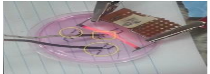
Fig. 21: Marked 10cm cell culture dish placed under a flat strip IR source
