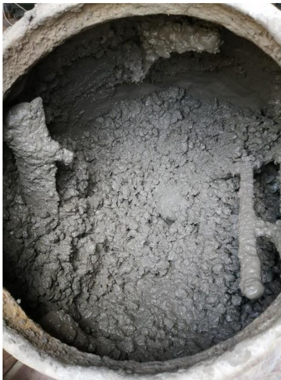
Fig.3: Concrete after mixing in the pan mixer
