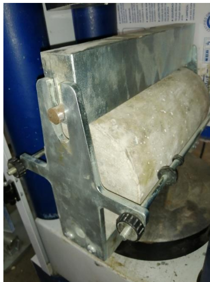
Fig.5: The setup of tensile splitting strength testing
