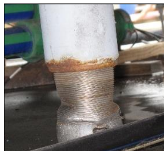
(b) Telescopic buckling: 2.8% in 2013 (<1.0% in 2016)
