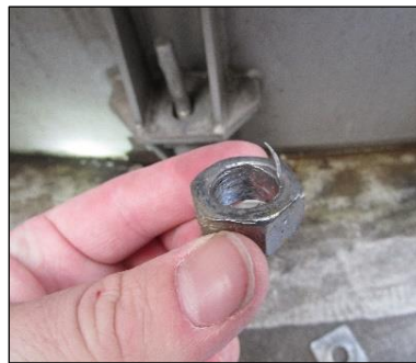
(b) Thread shearing: 7.5% in 2013 (4.0% in 2016)
