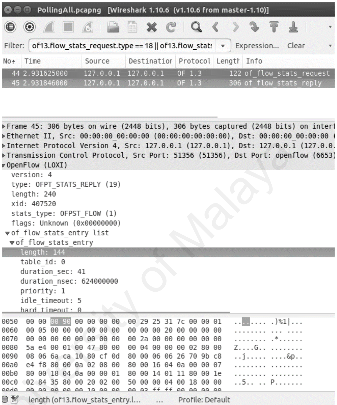
Figure 3.4: Request and reply message in PA approach in out-of-band network deployment.
