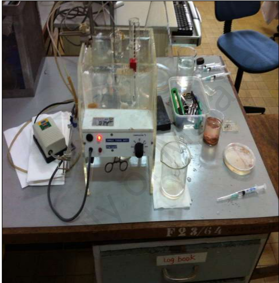
Figure 4.1: Organ bath connected to the Powerlab Programme.
