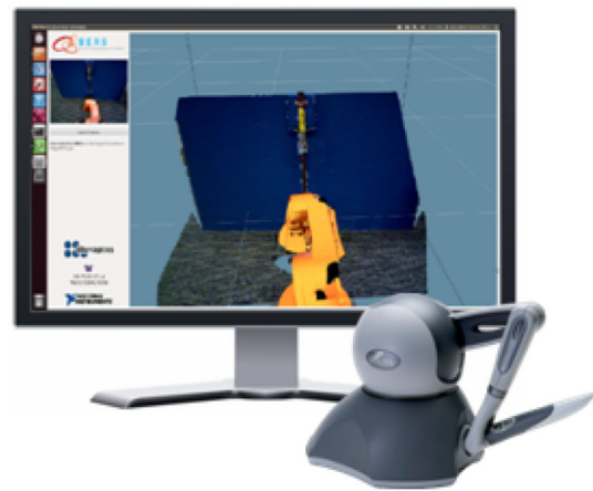
Fig. 1 Teleoperation master console station. Includes 3DOF haptic device as well as a LCD monitor to display visual feedback
