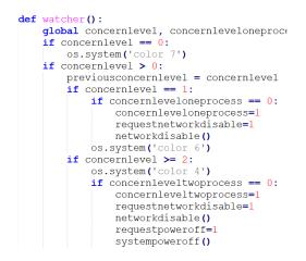
Figure 22: The "watcher" function (source code)
