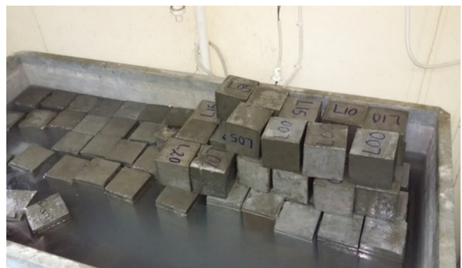
Fig. 2. Some of cubes and prisms during curing.
