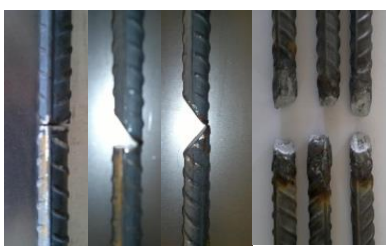
Prepared/failure bars in G6
