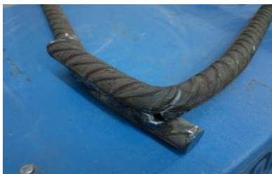
Crack/bond failure in bend test
