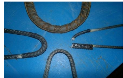
pass/fail specimens-bend test
