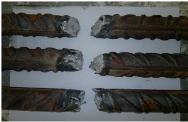
Failures of G2 25mm bars
