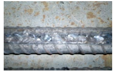
Fillet weld, V-flare lap joint
