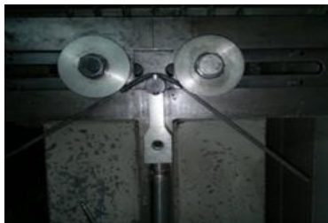
Lapped 8mm in bend test
