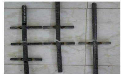
Failure planes for G4
