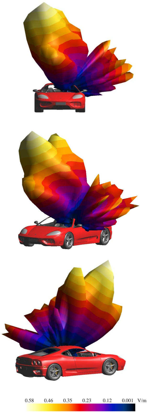
Fig. 11. Different views of the 3D total electric radiation pattern of the handset in hand close proximity to head at cheek-position while making a mobile call inside a car.
