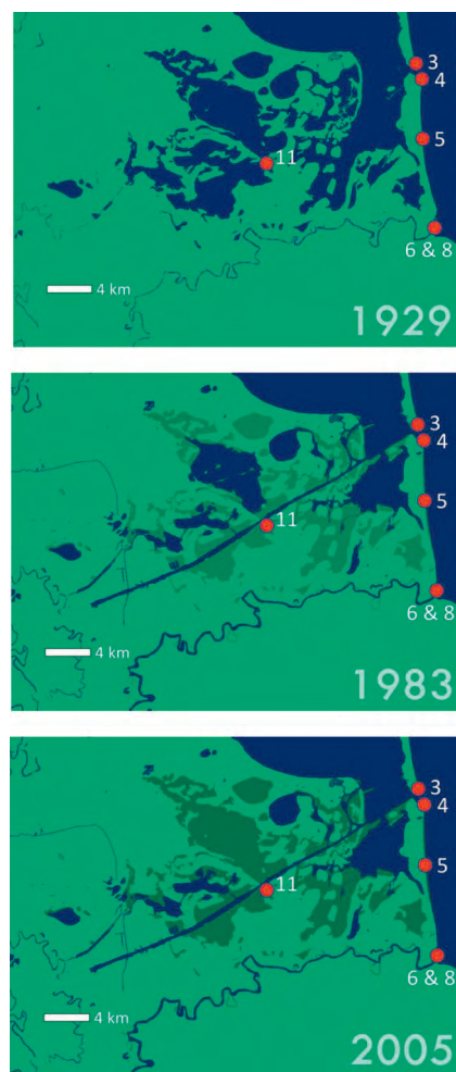
Figure 3. Morphological change of the Rio Grande delta system related to anthropogenic activity. Locations of samples #3–#8 and #11 shown: (A) Delta wetland region in 1929 prior to most dam construction; (B) 1983 conditions after creation of the Brownsville ship channel and construction of jetties and dredging of Brazos Santiago Pass; (C) 2005 conditions after continued dredging and draining of delta wetlands.
